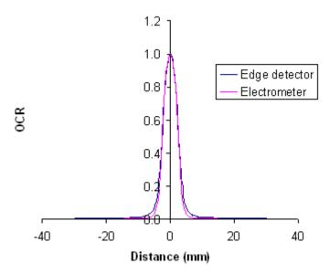
➤ Average of the root mean square deviation between the two detectors is 0.15 mm
